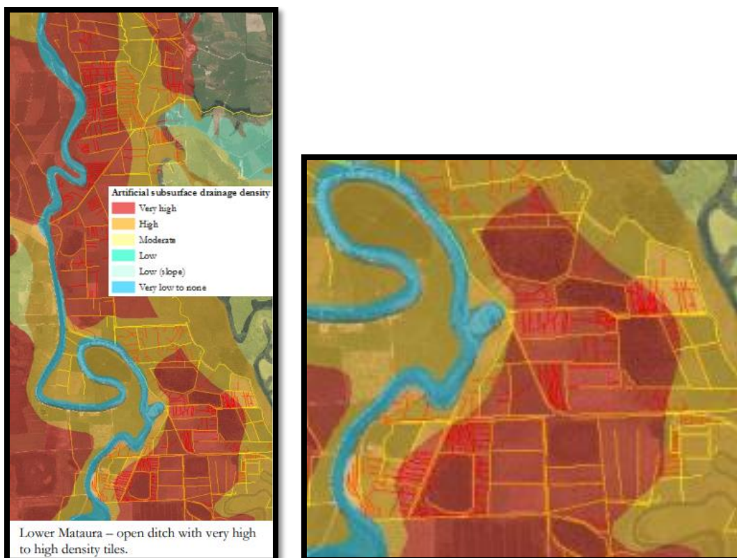
Figure 3 – Lower Matura River - Open ditch drainage network (yellow lines) with known tile (sub-surface) locations (red lines). 16
