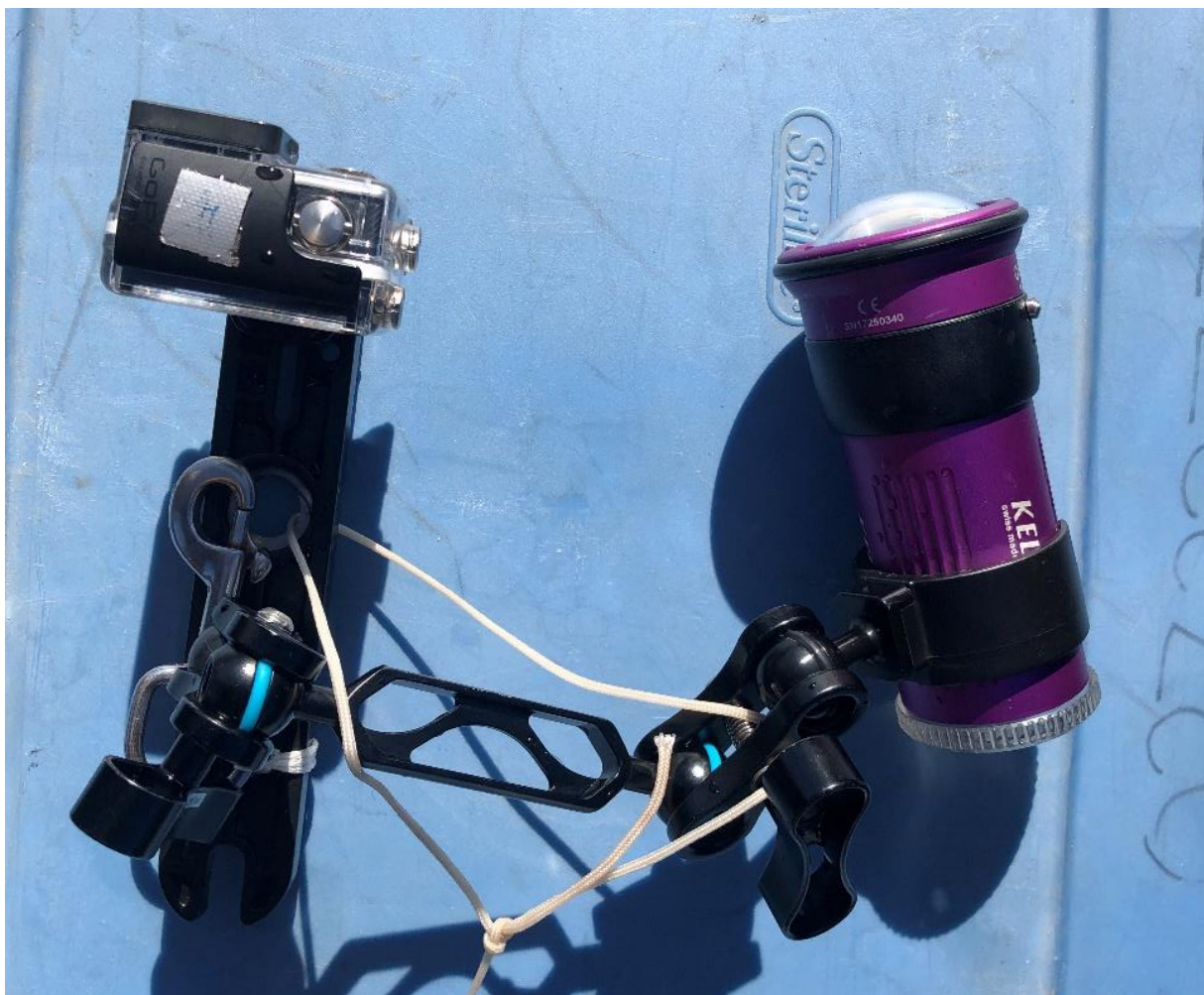
Figure 2-2: Drop camera system consisting of a GoPro Hero4 camera and associated dive torch.
